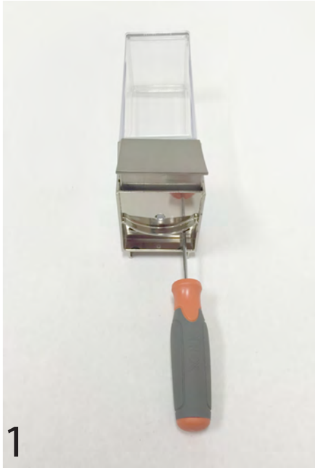
1. Remove 2 screws with a Phillips head screwdriver.
